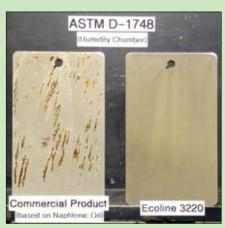
EcoLine® 3220 provides long lasting vapor corrosion inhibition and is made from renewable materials. Here is EcoLine® 3220 tested in comparision to another commercial product.
